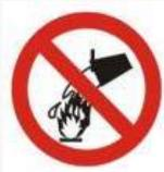
***IT IS STRICTLY PROHIBITED*** to fight any fire at the generator and machine using water or other liquid.
