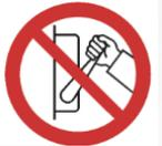
***IT IS PROHIBITED to turn on the machine by workers without being previously trained in service and Industrial Safety regulations.***
