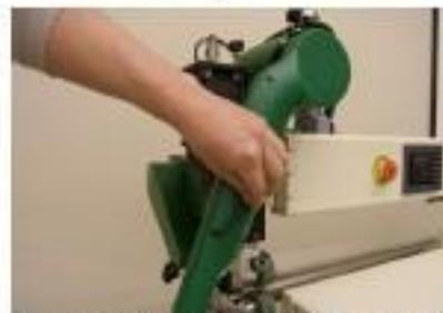
3. Loosen and remove the housing cover.
