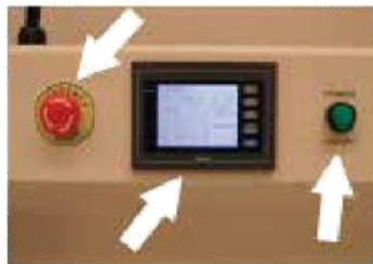
Control Panel, Power on-off Emergency Stop
