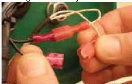
4. Disconnect the male from the female leads..
