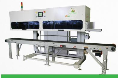
Seal Type: Pinch Closure and Double Fold Closure
