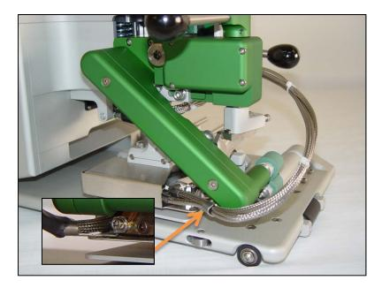
Install wedge on wedge mount arm using two screws.
