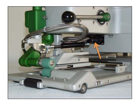
Electrically connect hot wedge to receptacle on body of Triad. When connected, make comfortable bend of heater wire and position properly in clip. Swing wedge in and out of welding position to make sure wrap around back of Triad is comfortable. When completed, tighten clip to secure.
