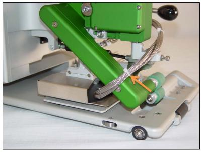
With wedge in engaged position, use zip ties to collect heater wires together. Note the wrap of heater wires around upper pinch roller arm and around back of Triad.
