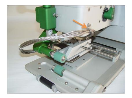
Using clip & screw, attach around heater wires and position to body of Triad. Do not fully tighten.
